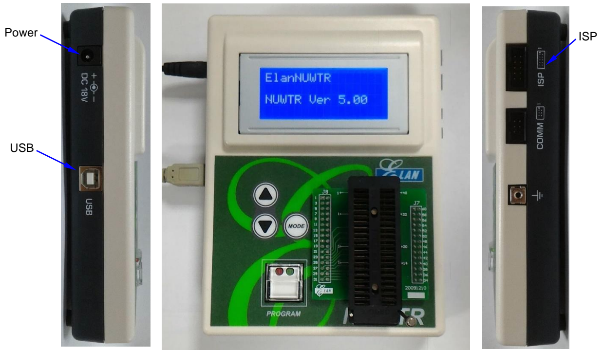
Figure D-1 Connecting NUWTR Writer to Host Computer (Left / Top / Right View)
